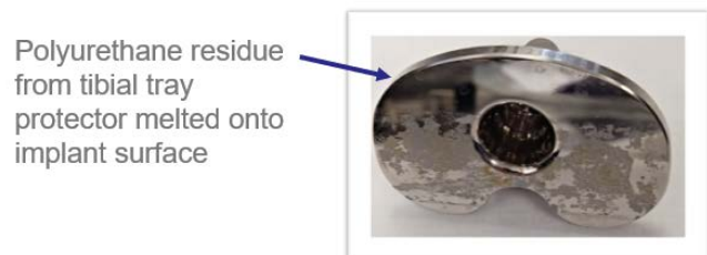
Image 2: Example of residual material on implant surface
