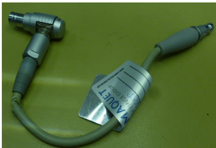
Figure 2: Example of torn cable insulation from the field
