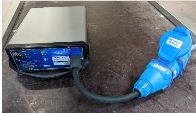
Figure 8 : Battery NiMH connected to NITE
