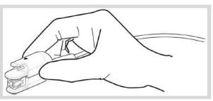
Figure 2-5: Grasping the Fiber-Optic sensor connector
