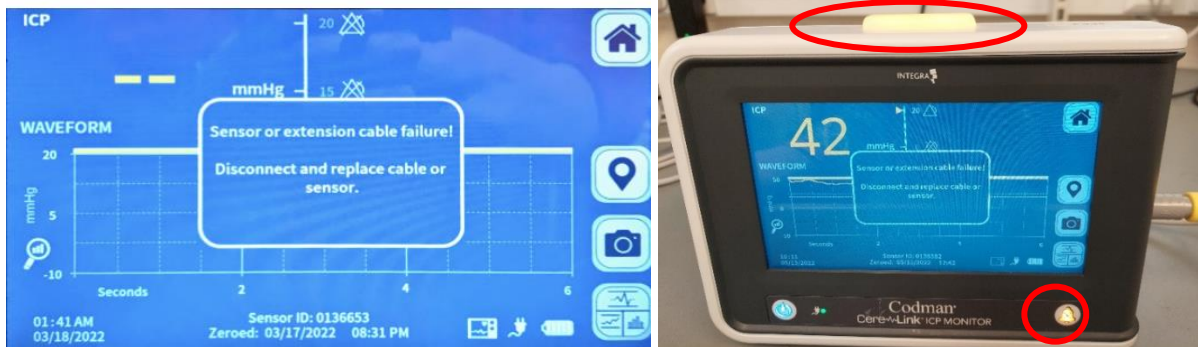
Figures 1 (left) and 2 (right): Visual alarms including display and flashing light alarm
