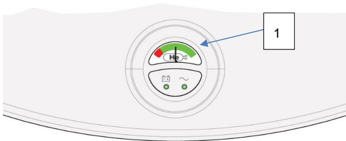
**Figure 2 – Top Panel (1 – Mechanical Helium Gauge)**
