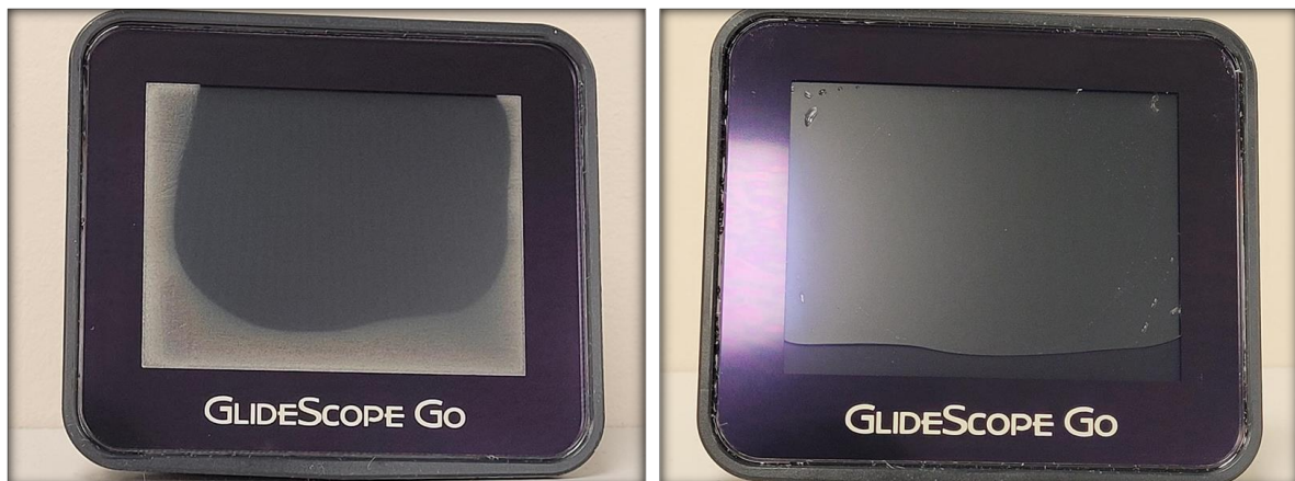
Figures 1 and 2: Representative images of fluid ingress seen in GlideScope Go monitors
