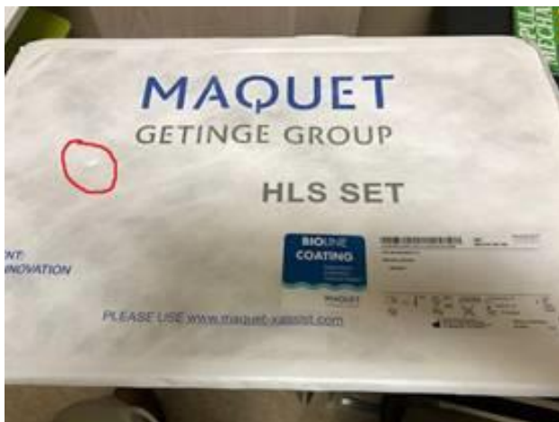
Picture 3 : HLS Set – defects in Tyvek
