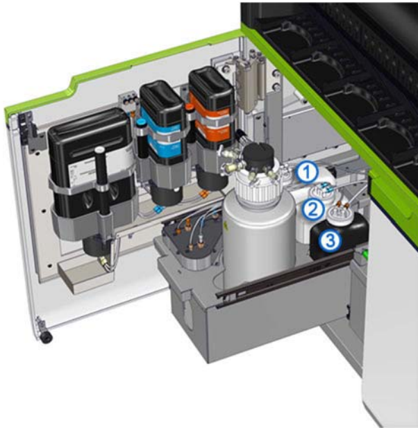
Bulk solution reservoir components (Alinity i)
